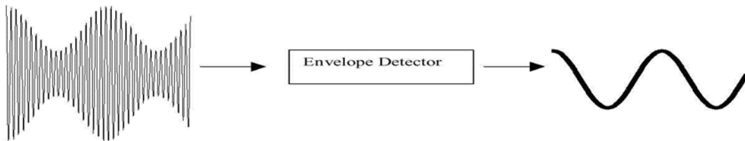
Figure 8-8 Demodulation of AM Signal
