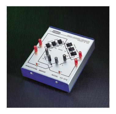
flow through the galvanometer, see if you can bring the bridge into balance without a range change. If a range change is necessary, do it one step at a time and again try to balance the bridge.
