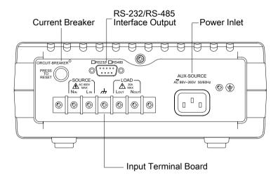
\*\*Current Breaker: This is an Over-current protected component. When the measurement is interrupted with over current input, please reduce the measured load, then re-switch on, the measurement can be back to normal.
