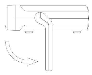
2). Pull apart the handle from the Power Meter. Please turn the handle left and right side slightly, that will make it easier to pull off the handle.
