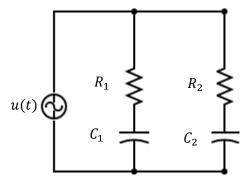
Let  $x_1(t)$  denote the voltage across capacitor  $C_1$  and  $x_2(t)$  denote the voltage across  $C_2$  at time t. The input to this circuit is a voltage source, where u(t) denotes the voltage input at time t. Suppose you have two sensors to measure the voltage drops across the resistors  $R_1$  and  $R_2$ , respectively.
